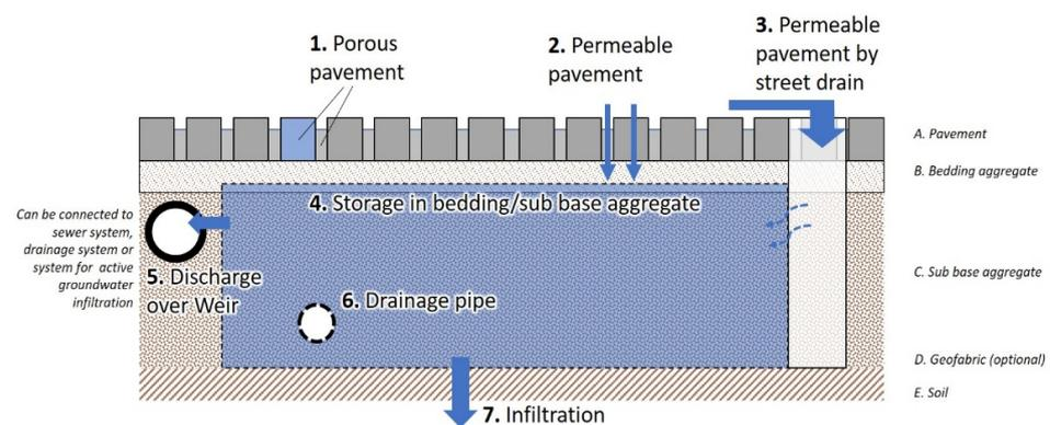
Figure 1. Classification of working principles in permeable systems.
