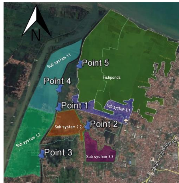
Figure 16, all sub systems where a water level difference is measured are shown. The fishponds are part of sub system 4.1. The points on the map are the points where a difference in water level is measured between the sub systems and the river
