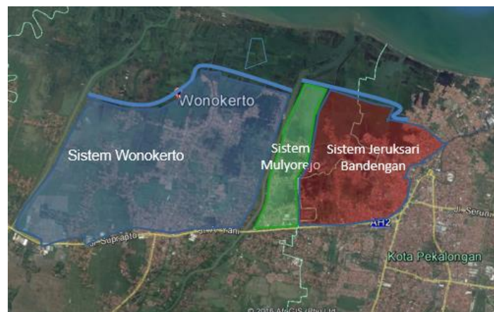
Figure 32, 3 sub systems (polders) which will be protected by a levee in the North. Border between kota and kabupaten is shown green. It is unclear if the blue and green areas will be built in the future.
