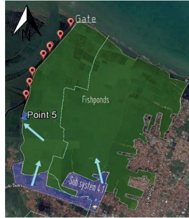
Figure 22, drainage using gravity is possible when the gate is closed. The blue arrows show that water could be drained to the fishponds and canal Bremi
