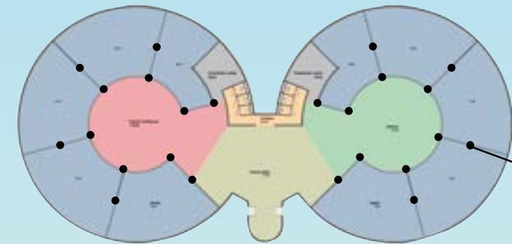
Reduction from 32 to 12 supporting columns (per tank). A relatively low cost adjustment to create a more open plan design giving this function more space as well as flexibility for other (more relevant) functions in the future
